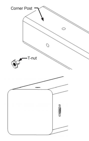
This picture shows the T-nut inserted and installed flush to the wood.
