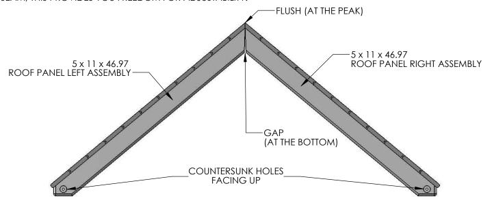
3: PLACE THE FRONT PLASTIC ARCH ON TOP OF THE ROOF SUPPORTS. MAKE SURE TO KEEP THE ROOF PANEL ASSEMBLIES TIGHT AT THE PEAK AND THE FRONT PLASTIC ARCH FLUSH TO THE ROOF OVERHANG ON BOTH SIDES. FASTEN USING #8 X 1-1/4" WOOD SCREWS. THE FINAL ASSEMBLY SHOULD MEASURE 69-7/8" AT THE BOTTOM.
