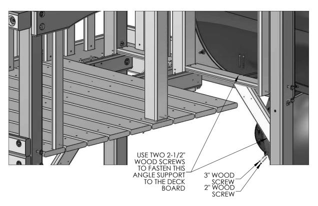
3: FOR THE 2 X 4 X 18" ANGLE SUPPORTS AT THE RIGHT FRONT USE TWO2-1/2" WOOD SCREWS THROUGH THE DECK AND INTO THE ANGLE SUPPORT. USE ONE 2" AND ONE 3" WOOD SCREW TO FASTEN THE RIGHT FRONT ANGLE SUPPORTS TO THE RIGHT FRONT CORNER POST.
