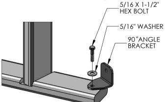
7: INSTALL THE 90° ANGLE BRACKETS TO THE INSIDE OF THE LADDER RAILS WITH 5/16 X 1-1/2" BOLTS, 5/16 WASHERS, INTO THE 5/16" T-NUTS.
