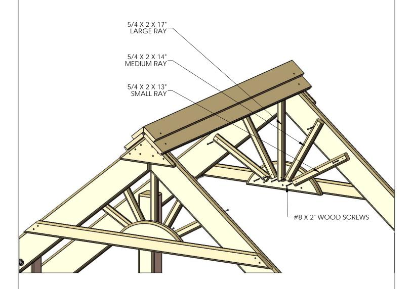
NOTE: ROOF BOARDS AND OTHER DETAILS OMITTED FOR CLARITY.
