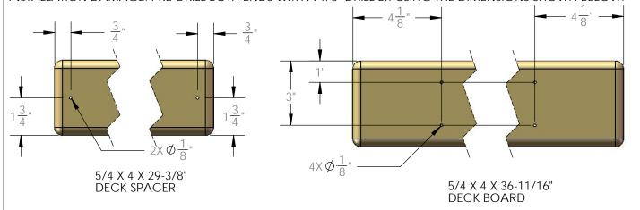
2: PLACE THE  $5/4 \times 4 \times 29$ -3/8" DECK SPACERS BETWEEN THE CORNER POSTS. MAKE EACH DECK SPACER FLUSH TO THE INSIDE SURFACE OF THE 2 X 6 OR THE OUTSIDE SURFACE OF THE CORNER POSTS. DO NOT ATTACH THE DECK SPACERS YET.
