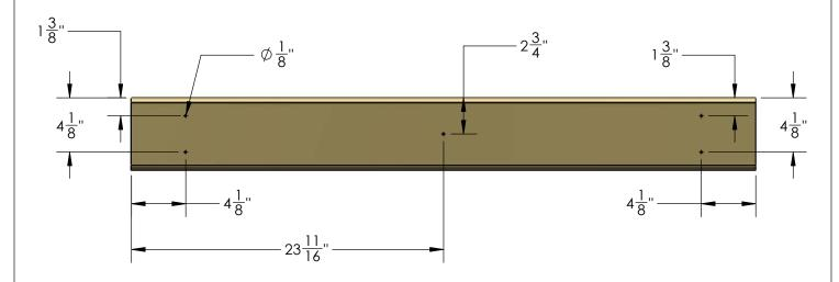
2: START WITH A 5/4 X 6 X 47-3/8" DECK BOARD AT ONE END OF THE FORT. CENTER THE BOARD BETWEEN THE FRONT FACE BOARD AND THE REAR BOTTOM PANEL BOARD AND ATTACH IT WITH 2" WOOD SCREWS THROUGH THE PREDRILED HOLES AND INTO THE DECK SUPPORT BELOW. LEAVE A UNIFORM (APPROX. 1/4") SPACE BETWEEN THE DECK BOARDS. NOTE: THE TOP OF THE SCREW HEAD SHOULD BE FLUSH TO THE TOP OF THE DECK BOARDS.
