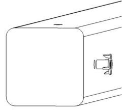
Insert the barrel of the T-nut into the predrilled hole. Using a smooth faced hammer, drive the T-nut until the face of the T-nut is flush to the wood.
