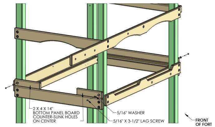
2: PLACE THE 2 X 4 X 47-1/2" BOTTOM PANEL BOARD ON TOP OF THE 2 X 6 PANEL BOARD WITH OFFSET HOLES UPAND FASTEN TO THE CORNER POSTS WITH 5/16" X 3-1/2" LAG SCREWS AND 5/16" WASHERS.
