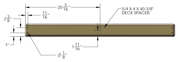
2: PLACE THE 5/4 X 4 X 40-3/8" DECK SPACER AT ONE END OF THE FORT. CENTER THE BOARD BETWEEN THE CORNER POSTS AND ATTACH IT WITH 2" WOOD SCREWS THROUGH THE PREDRILLED HOLES INTO THE DECK SUPPORT BELOW. NOTE THE TOP OF THE SCREW HEAD SHOULD BE FLUSH TO THE TOP OF THE DECK SPACER.
