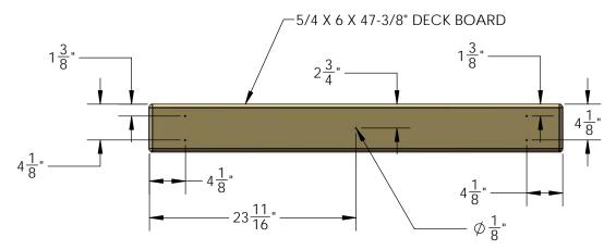
2: START WITH A 5/4 X 6 X 47-3/8" DECK BOARD AT ONE END OF THE FORT. CENTER THE BOARD BETWEEN THE FRONT FACE BOARD AND THE REAR BOTTOM PANEL BOARD AND ATTACH IT WITH 2" WOOD SCREWS THROUGH THE PREDRILED HOLES AND INTO THE DECK SUPPORTS BELOW. LEAVE A UNIFORM (APPROX. 1/4") SPACE BETWEEN THE DECK BOARDS. NOTE: THE TOP OF THE SCREW HEAD SHOULD BE FLUSH TO THE TOP OF THE DECK BOARDS.
