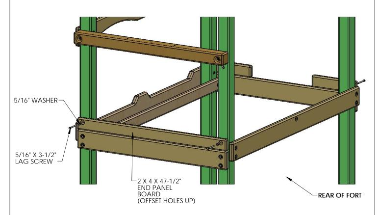
1: PLACE THE 2 X 4 X 14" BOTTOM PANEL BOARD ON TOP OF THE 2 X 6 PANEL BOARD AND FASTEN TO THE CORNER POSTS WITH 5/16" X 3-1/2" LAG SCREWS WITH 5/16" WASHERS.
