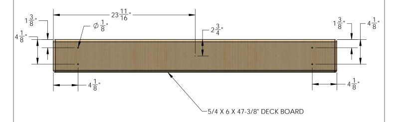
2: START WITH A 5/4 X 6 X 47-3/8" DECK BOARD AT ONE END OF THE FORT. CENTER THE BOARD BETWEEN THE FRONT FACE BOARD AND THE REAR BOTTOM PANEL BOARD AND ATTACH IT WITH 2" WOOD SCREWS THROUGH THE PREDRILLED HOLES AND INTO THE DECK SUPPORT BELOW. LEAVE A UNIFORM (APPROX. 1/4") SPACE BETWEEN THE DECK BOARDS. NOTE: THE TOP OF THE SCREW HEAD SHOULD BE FLUSH TO THE TOP OF THE DECK BOARDS.
