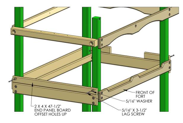
2: PLACE THE 2 X 4 X 14" BOTTOM PANEL BOARD ON TOP OF THE 2 X 6 PANEL BOARD AND FASTEN TO THE CORNER POSTS WITH 5/16 X 3-1/2" LAG SCREWS WITH 5/16" WASHERS.
