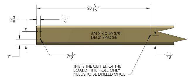
2: PLACE THE 5/4 X 4 X 40-3/8" DECK SPACER AT ONE END OF THE FORT. CENTER THE BOARD BETWEEN THE CORNER POSTS AND ATTACH IT WITH 2" WOOD SCREWS THROUGH THE PREDRILLED HOLES AND INTO THE DECK SUPPORT BELOW. NOTE THE TOP OF THE SCREW HEAD SHOULD BE FLUSH TO THE TOP OF THE DECK SPACER.
