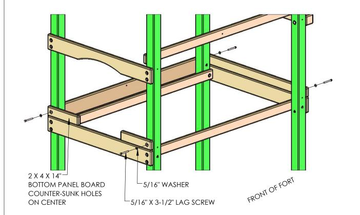
2: PLACE THE 2 X 4 X 47-1/2" BOTTOM PANEL BOARD (HOLES OFFSET UP) ON TOP OF THE 2 X 6 PANEL BOARD AND FASTEN TO THE CORNER POSTS WITH 5/16" X 3-1/2" LAG SCREWS AND 5/16" WASHERS.
