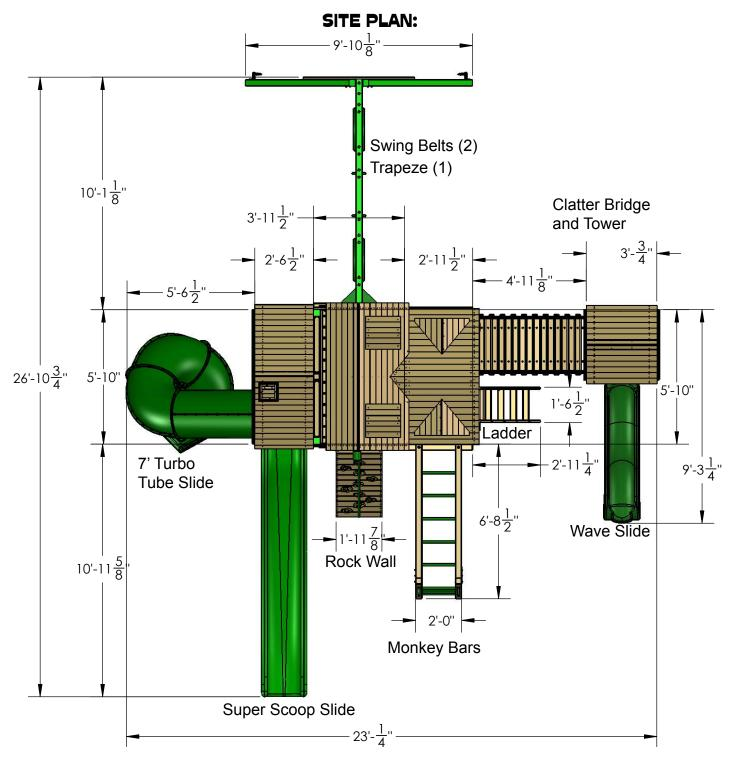
Playset height: 13 feet - 1-5/8 inches Deck heights: 4 feet, 5 feet and 7 feet Swing Beam height: 7 feet - 7-1/2 inches
