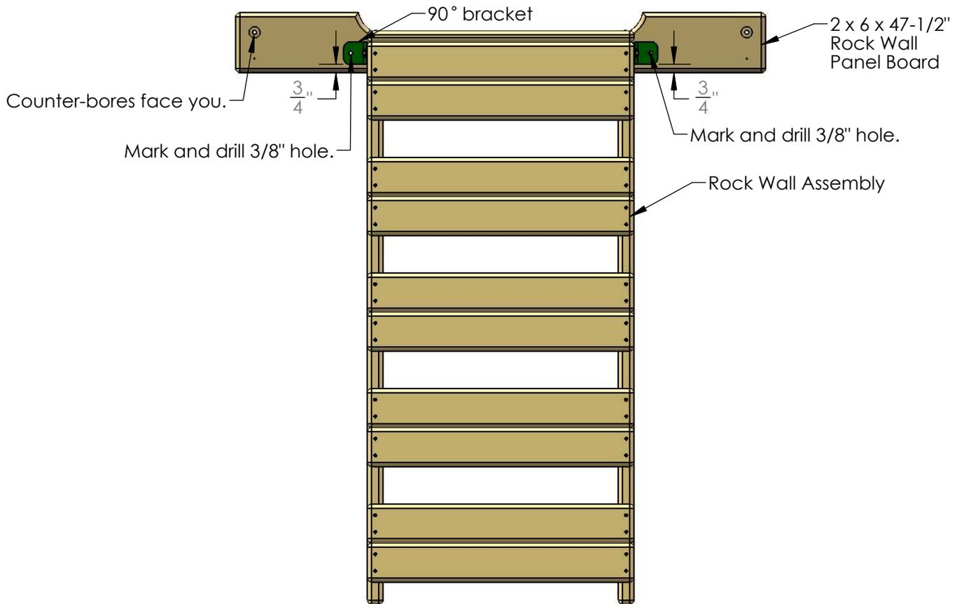
3: Now flip the Rock Wall Panel Board over and install a T-nut into each of the holes you just drilled. Place the Rock Wall Panel Board and the Rock wall aside for use in a later step.
