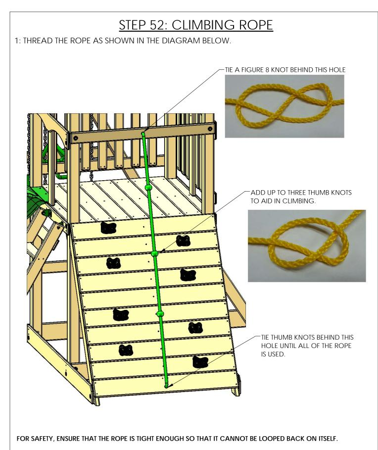
KEEP TYING THUMB KNOTS AT THE BOTTOM END OF THE ROPE UNTIL THERE IS NO REMAINING LOOSE ROPE.
