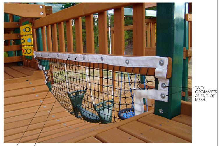
CENTER THE MESH PANEL ON THE CLATTER BRIDGE RAIL ON THE INSIDE. NOTE THE GROMMETS HAVE A RECESSED PART ON ONE SIDE AN IT SHOULD FACE YOU.
