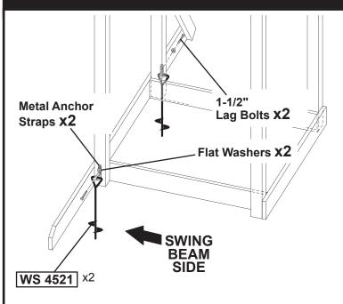
Install stakes into 3 x 3" uprights. Locate stakes as shown.
