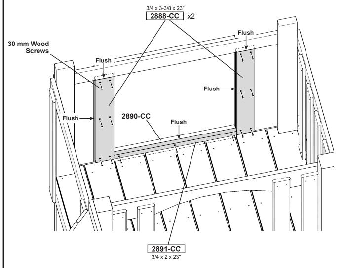
Insert 2891-CC between deck boards and 2890-CC. Secure with (3) 30 mm screws.
