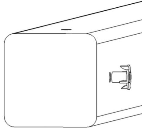
Insert the barrel of the T-nut into the predrilled hole. Using a smooth faced hammer, drive the T-nut until the face of the T-nut is flush to the wood.
