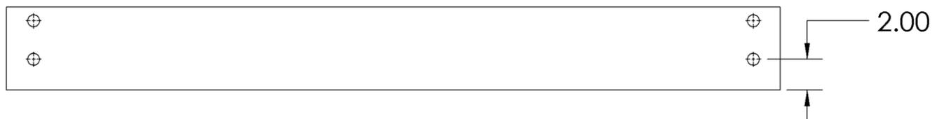
**Counter-sunk holes-** Many of the parts that will be used have counter-sunk holes. A counter-sunk hole is one that surrounds one side of a thru hole, but does not extend through the wood itself. When using a counter-sunk hole the bolt will be inserted through the thru hole and either the head of the bolt and washer or nut and washer will occupy the counter sunk hole.
