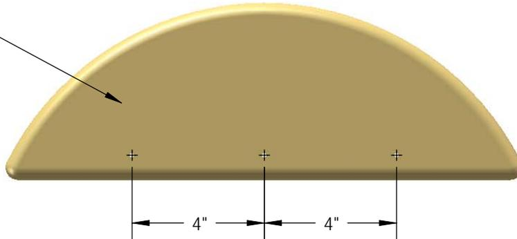
2: PLACE THE 2 X 6 X 16" SUN CENTERED AGAINST THE 5/4 X 2-5/8 X 42" SUN SUPPORT. FASTEN THE SUN TO THE SUN SUPPORT WITH 2" WOOD SCREWS.
