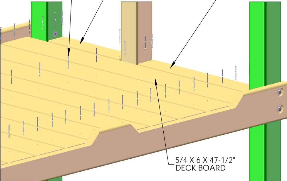
2: START WITH A 5/4 X 6 X 47-1/2" DECK BOARD AT ONE END OF THE FORT. CENTER THE BOARD BETWEEN THE FRONT FACE BOARD AND THE REAR BOTTOM PANEL BOARD AND ATTACH IT WITH 2" WOOD SCREWS THROUGH THE PREDRILED HOLES AND INTO THE DECK SUPPORT BELOW. LEAVE A UNIFORM (APPROX. 1/4") SPACE BETWEEN THE DECK BOARDS. NOTE: THE TOP OF THE SCREW HEAD SHOULD BE FLUSH TO THE TOP OF THE DECK BOARDS.
