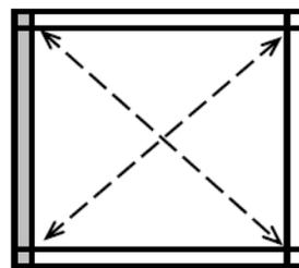
The diagonal measurements should be the same from corner post to corner post. If not, adjust corner posts so that the distance is equal.
