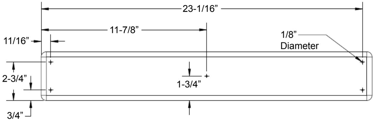
2: Four 5/4 x 4 x 23-3/4" Deck Spacers will fit at each end of the deck between the Corner and Center Posts. Attach the Deck Spacers with 2" wood screws through the pre-drilled holes.
