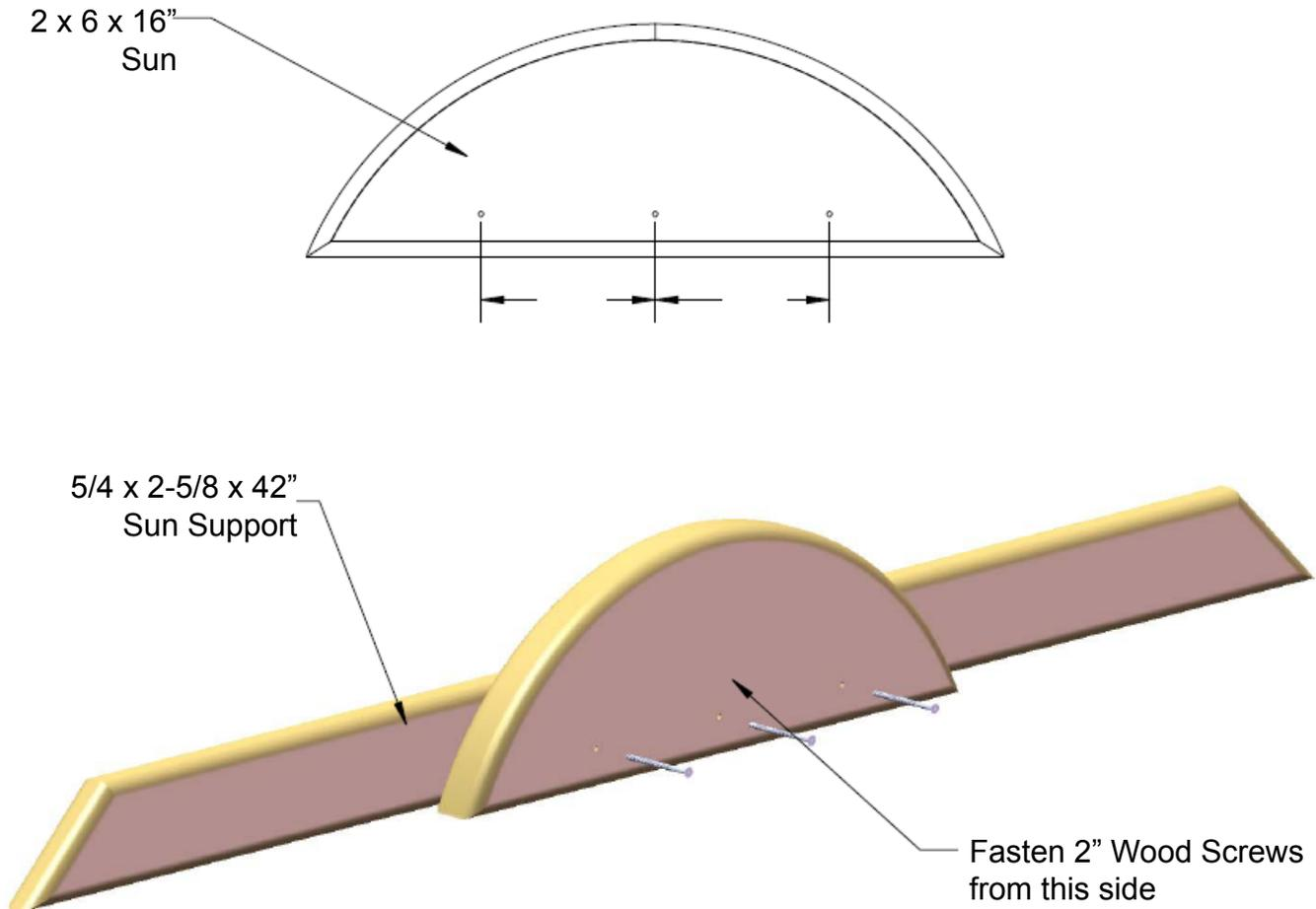
**Note: The top of the screw head should be flush to the surface of the Sun.**
