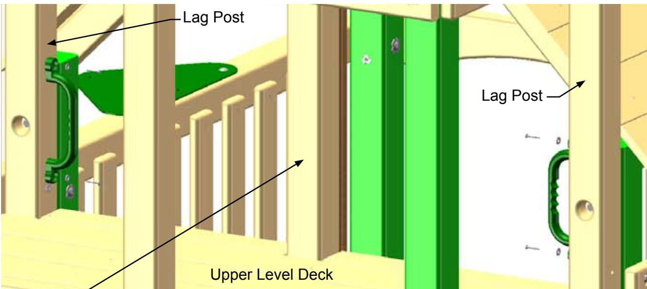
Upper Level Front Center Post (Alternate place mount to Safety Handles.)
