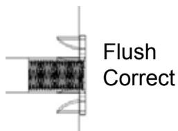
Cross Section end views, you are looking at an Xray view of the post and T-nut. The barrel of the T-nut is in the corner post the line is the face of the wood.
