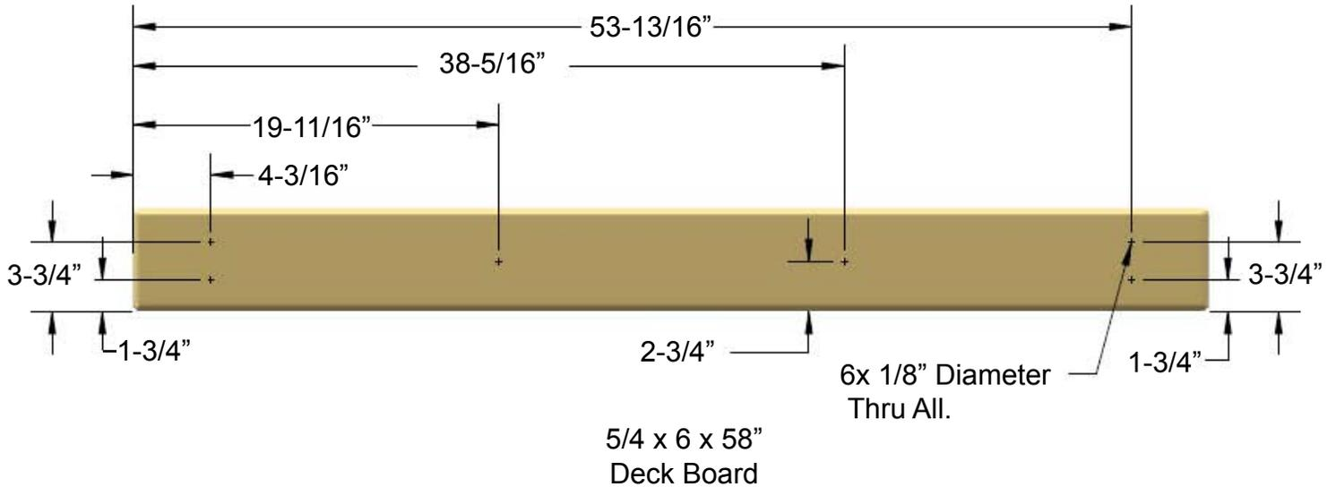
2: Start with a 5/4 x 6 x 58" Deck Board at one end of the fort. Center the Deck Board between the Side Face Board and the Bottom Panel Board and attach it with 2" wood screws through the pre-drilled holes and into the Deck Support below. Leave a uniform (about 1/4") space between the Deck Boards. Note: The top of the screw head should be flush to the top of the Deck Boards.
