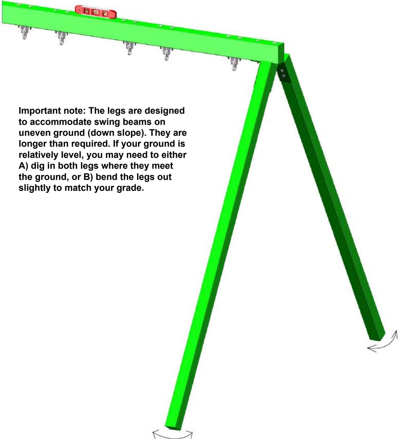
**Important note:** The legs are designed to accommodate swing beams on uneven ground (down slope). They are longer than required. If your ground is relatively level, you may need to either A) dig in both legs where they meet the ground, or B) bend the legs out slightly to match your grade.
