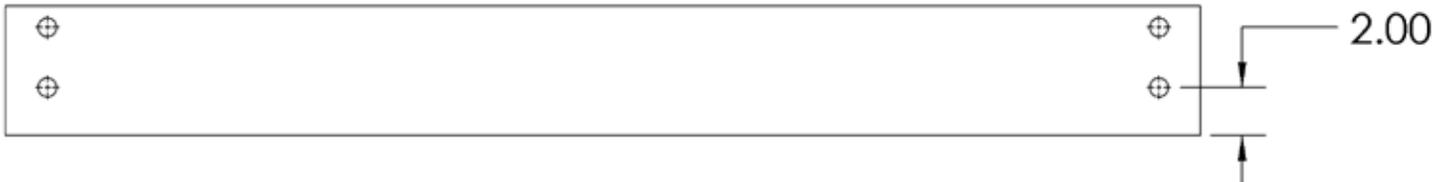
**Counter-sunk holes-** Many of the parts that will be used have counter-sunk holes. A counter-sunk hole is one that surrounds one side of a thru hole, but does not extend through the wood it's self. When using a counter-sunk hole the bolt will be inserted through the thru hole. In some cases the bolt head with a washer will occupy the counter-sunk hole. In other cases a nut with a washer will occupy the counter-sunk hole.
