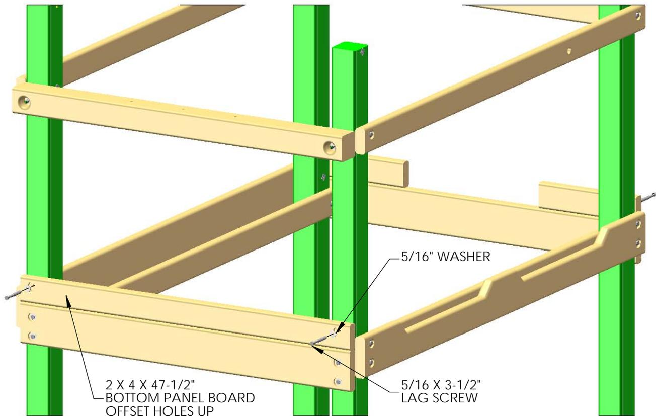
2: PLACE THE 2 X 4 X 14" BOTTOM PANEL BOARD ON TOP OF THE 2 X 6 PANEL BOARD, AND FASTEN TO THE CORNER POSTS WITH 5/16 X 3-1/2" LAG SCREWS WITH 5/16" WASHERS.
