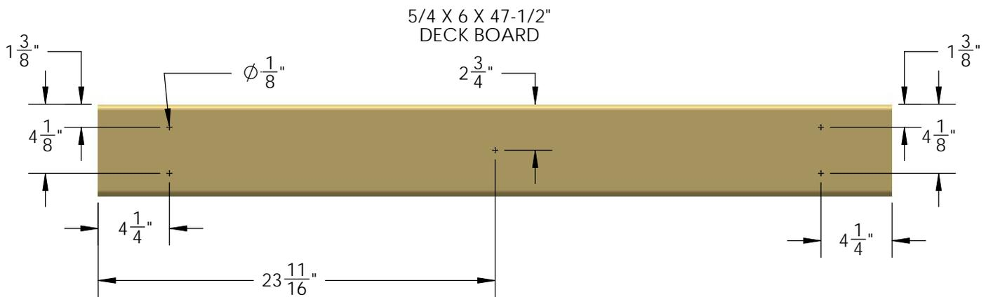
2: START WITH A 5/4 X 6 X 47-1/2" DECK BOARD AT ONE END OF THE FORT. CENTER THE BOARD BETWEEN THE FRONT FACE BOARD AND THE REAR BOTTOM PANEL BOARD AND ATTACH IT WITH 2" WOOD SCREWS THROUGH THE PREDRILLED HOLES AND INTO THE DECK SUPPORT BELOW. LEAVE A UNIFORM (APPROX. 1/4") SPACE BETWEEN THE DECK BOARDS. NOTE: THE TOP OF THE SCREW HEAD SHOULD BE FLUSH TO THE TOP OF THE DECK BOARDS.
