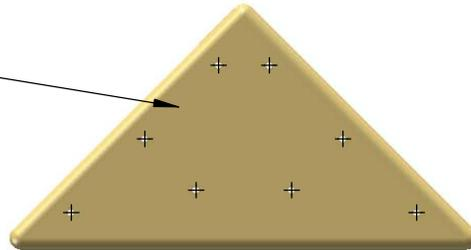
2: PLACE THE 5/4 X 10" ROOF PEAK SUPPORT AGAINST THE ANGLED ROOF SUPPORTS AND FLUSH TO THE SIDES OF THE ANGLED ROOF SUPPORTS. FASTEN THE ROOF PEAK SUPPORT TO THE ANGLED ROOF SUPPORTS WITH 1-1/2" WOOD SCREWS. REPEAT ON OTHER SIDE.
