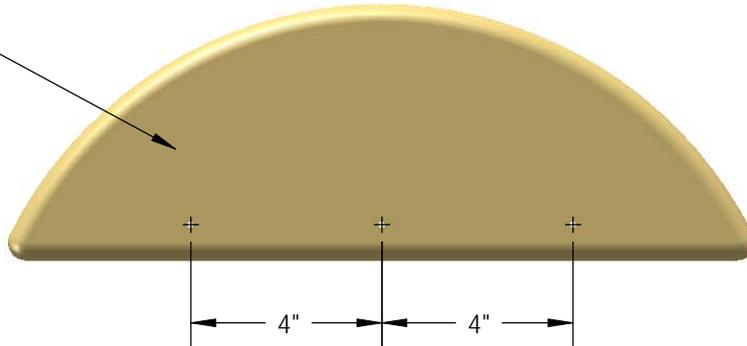
2: PLACE THE 2 X 6 X 16" SUN CENTERED AGAINST THE 5/4 X 2-5/8 X 42" SUN SUPPORT. FASTEN THE SUN TO THE SUN SUPPORT WITH 2" WOOD SCREWS. REPEAT THIS PROCESS FOR THE OTHER SIDE OF THE FORT.
