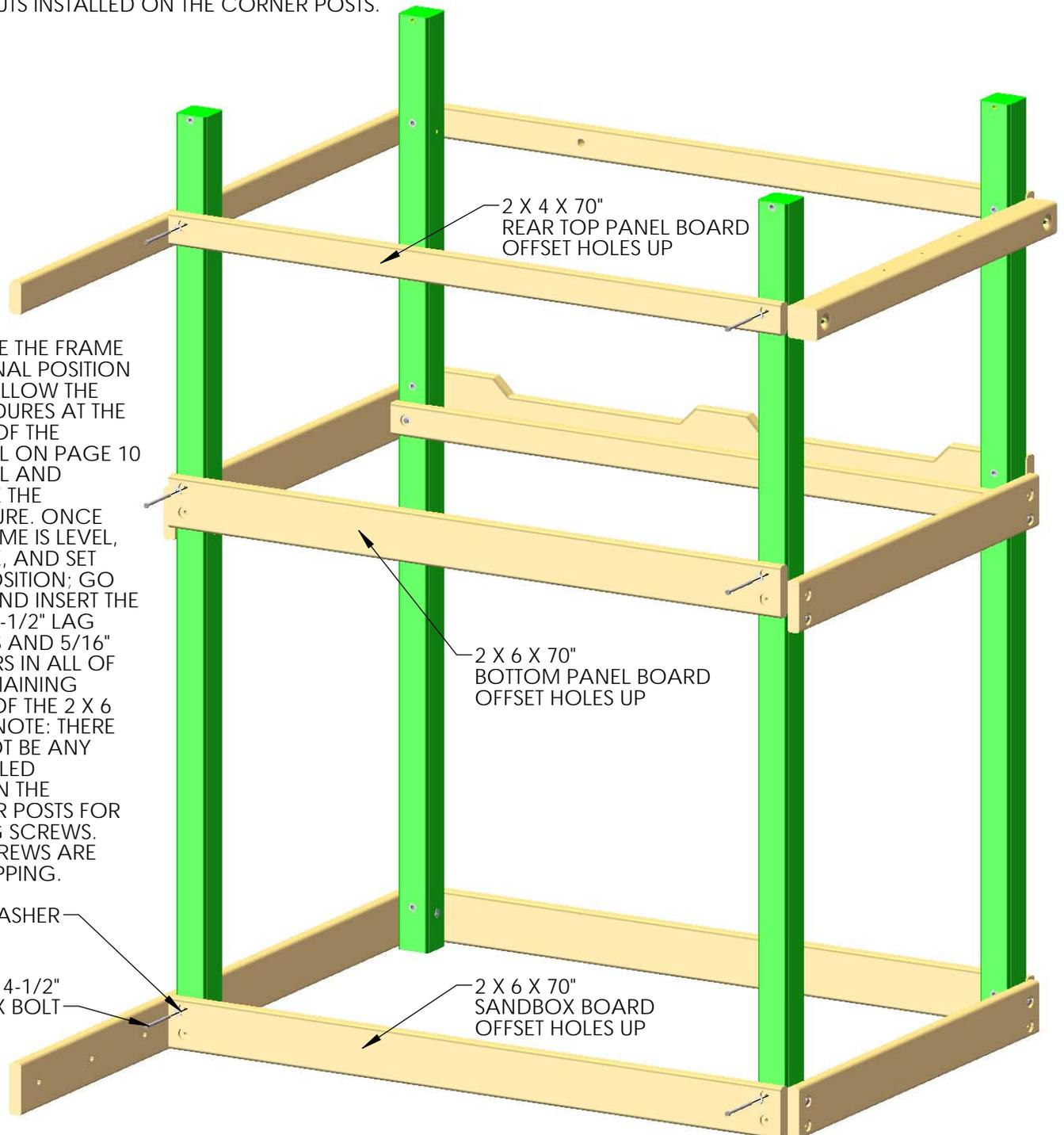
7: PLACE THE FRAME IN ITS FINAL POSITION AND FOLLOW THE PROCEDURES AT THE FRONT OF THE MANUAL ON PAGE 10 TO LEVEL AND SQUARE THE STRUCTURE. ONCE THE FRAME IS LEVEL, SQUARE, AND SET INTO POSITION; GO BACK AND INSERT THE 5/16 X 3-1/2" LAG SCREWS AND 5/16" WASHERS IN ALL OF THE REMAINING HOLES OF THE 2 X 6 PARTS. NOTE: THERE WILL NOT BE ANY PREDRILLED HOLES IN THE CORNER POSTS FOR THE LAG SCREWS. LAG SCREWS ARE SELF-TAPPING.
