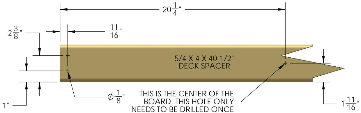
2: PLACE THE 5/4 X 4 X 40-1/2" DECK SPACER AT ONE END OF THE FORT. CENTER THE BOARD BETWEEN THE CORNER POSTS AND ATTACH IT WITH 2" WOOD SCREWS THROUGH THE PREDRILED HOLES AND INTO THE DECK SUPPORT BELOW. NOTE: THE TOP OF THE SCREW HEAD SHOULD BE FLUSH TO THE TOP OF THE DECK SPACER.
