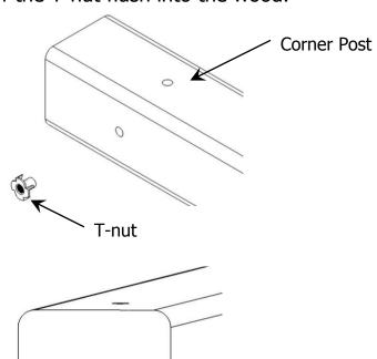
This picture shows the T-nut insert and installed flush to the wood.
