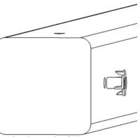
Insert the barrel of the T-nut into the predrilled hole. Using a smooth faced hammer, drive the T-nut until the face of the T-nut is flush to the wood.
