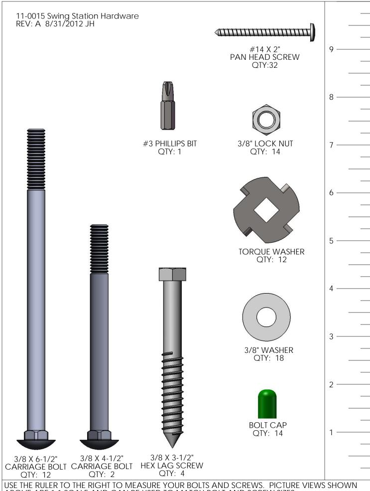
USE THE RULER TO THE RIGHT TO MEASURE YOUR BOLTS AND SCREWS. PICTURE VIEWS SHOWN ABOVE ARE 1:1 SCALE AND CAN BE USED TO MATCH BOLT AND SCREW SIZES.
