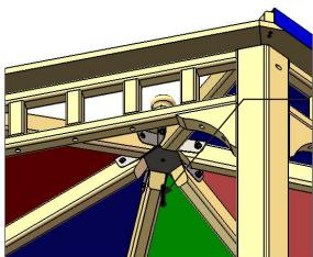
6mm x 55mm Phillips Pan head screw goes up through the bottom of the Apex bracket and screws into Roof Finial K
