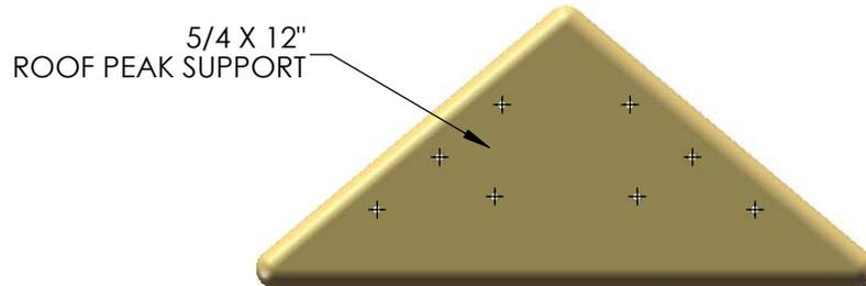
2: PLACE THE 5/4 X 12" ROOF PEAK SUPPORT AGAINST THE ANGLED ROOF SUPPORTS AND FLUSH TO THE SIDES OF THE ANGLED ROOF SUPPORTS. FASTEN THE ROOF PEAK SUPPORT TO THE ANGLED ROOF SUPPORTS WITH 1-1/2" WOOD SCREWS. REPEAT ON OTHER SIDE.
