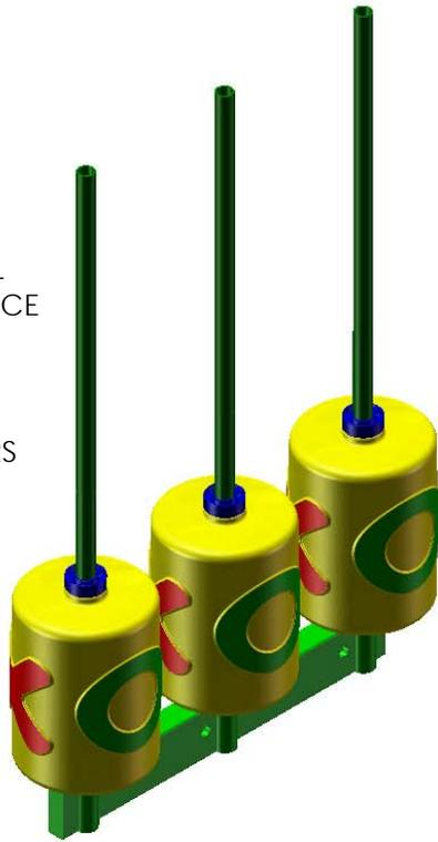
3: LOCATE THE GREEN BRACKET AND PLACE ON TOP OF ASSEMBLY. LINE UP THE HOLES IN THE BRACKET WITH THE DOWELS ON THE UNIT.
