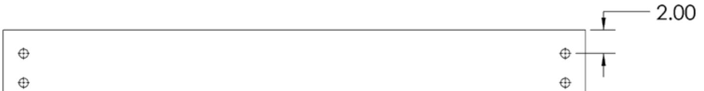
**Counterbored holes-** Many of the parts that will be used have counterbored holes. A counterbored hole is one that surrounds one side of a thru hole, but does not extend through the wood itself. When using a counterbored hole the bolt will be inserted through the thru hole. In some cases the bolt head with a washer will occupy the counterbored hole. In other cases a nut with a washer will occupy the counterbored hole.
