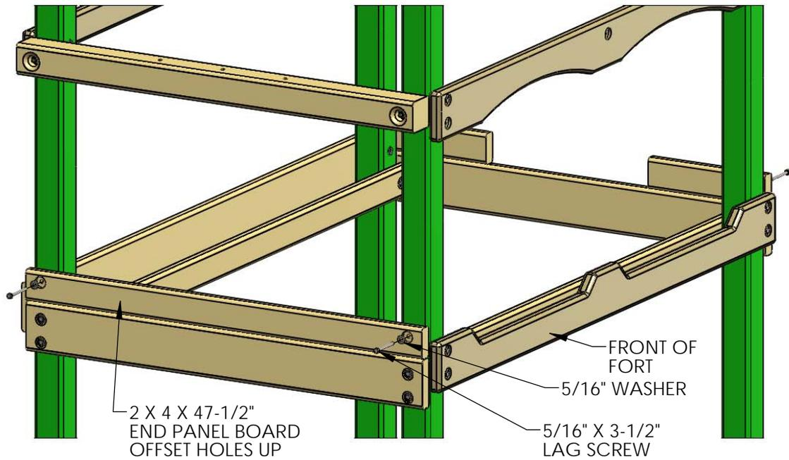
2: PLACE THE 2 X 4 X 14" BOTTOM PANEL BOARD ON TOP OF THE 2 X 6 PANEL BOARD AND FASTEN TO THE CORNER POSTS WITH 5/16 X 3-1/2" LAG SCREWS WITH 5/16" WASHERS.
