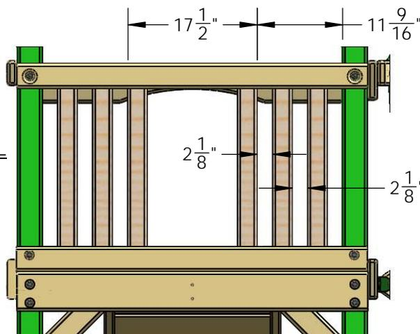
FRONT PANEL SLATS ARE INSTALLED FLUSH TO THE NOTCH ON THE FRONT FACE BOARD.
