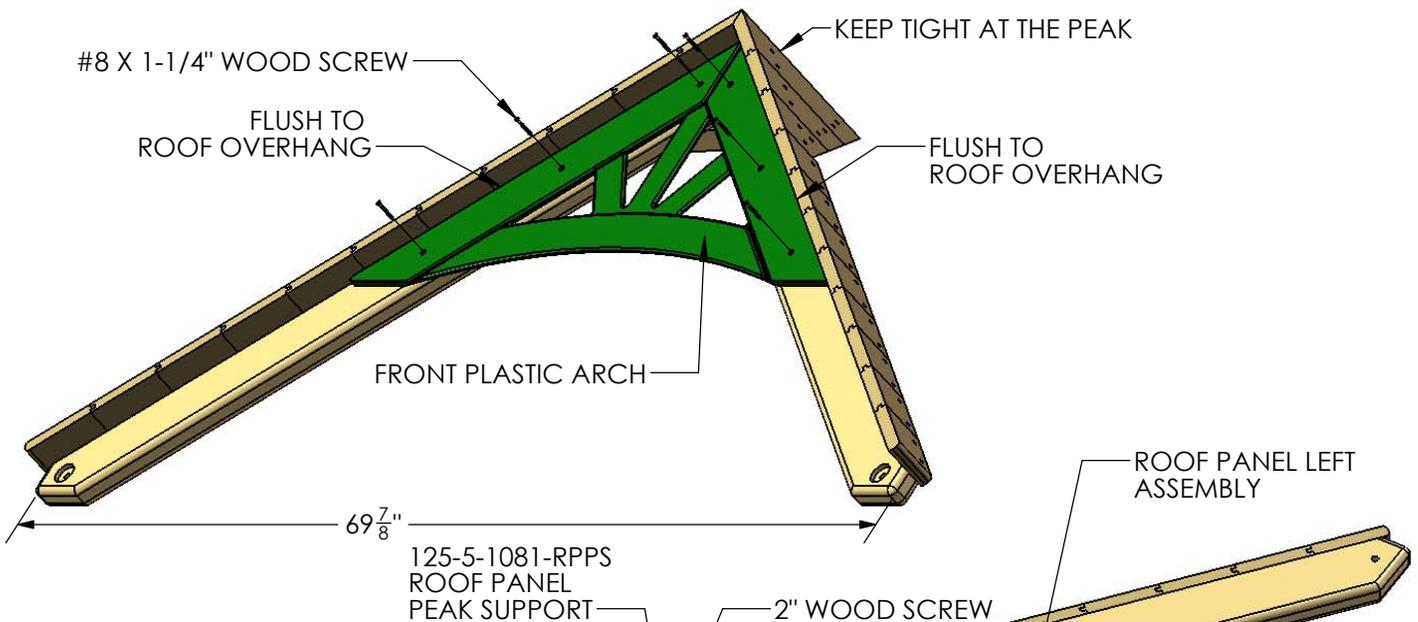
4: PLACE THE ROOF PANEL PEAK SUPPORT ON TOP OF THE TWO PANELS AND FLUSH TO THE SIDES OF THE ROOF BOARD BATTENS. FASTEN THE ROOF PANEL PEAK SUPPORT TO THE ROOF PANELS USING 2" WOOD SCREWS.
