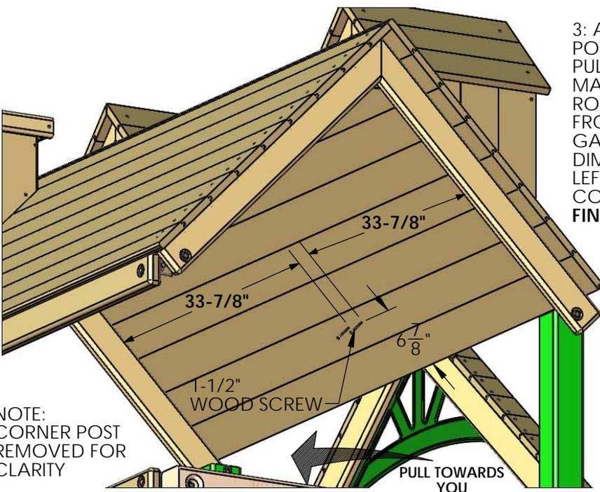
3: AFTER THE GABLE ASSEMBLY IS IN ITS FINAL POSITION. GO INSIDE ON TOP OF THE DECK AND PULL THE GABLE ASSEMBLY TOWARDS YOU MAKING SURE IT IS FLUSH TO THE OUTSIDE OF THE ROOF AND INSERT TWO 1-1/2" WOOD SCREW FROM UNDERNEATH THE ROOF INTO THE GABLE ASSEMBLY ROOF PEAK. USE THE DIMENSIONS SHOWN IN THE DIAGRAM TO THE LEFT TO INSERT THE WOOD SCREWS IN THE CORRECT LOCATION. **REMOVE THE ROOF FINISHERS, THESE WILL BE USED IN A LATER STEP.**
